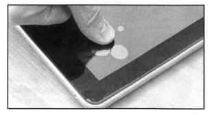
Push out any remaining bubbles for complete fit of the film
